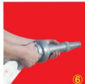
⑥ 对准火源根部，进行灭火 Aim at fire's root to put out fire
